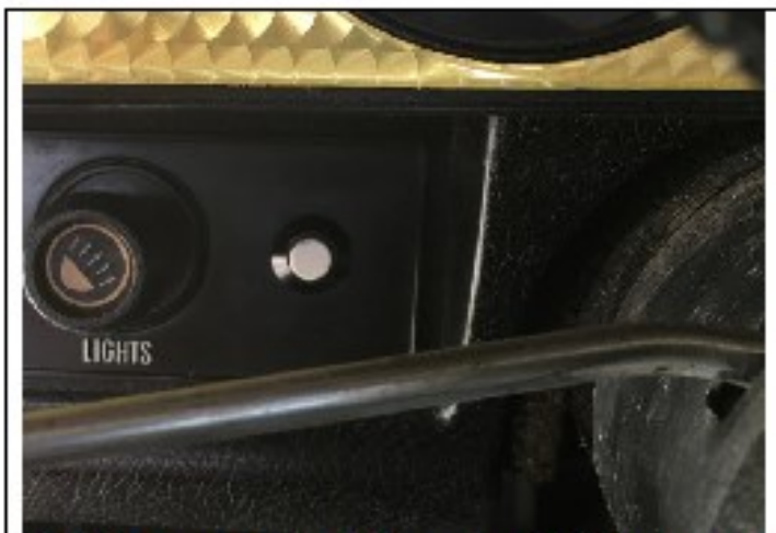
Push button to prime fuel pump added in place of the rear window defogger switch.
