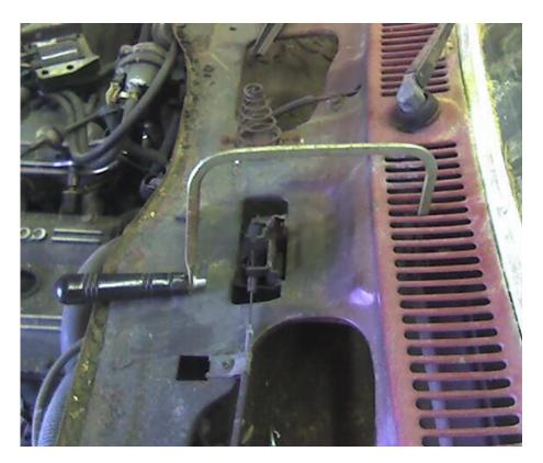
**Step 4.** Rotate the saw frame as shown below by inserting into the vertical "key hole" and angle it towards the driver's headlight. When you can pull the saw handle slightly towards yourself you will be able to feel the bottom V-tab.
