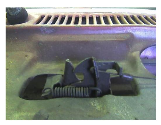
Here is the lower portion of the lock mechanism:
