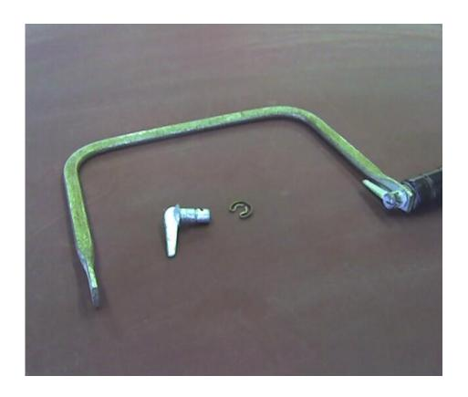
**Step 3.** Saw off the end and weld an extension approximately 1 inch lower that the side with the handle. Also, note the electrical tape on the top of the frame to protect your paint in the cowl vents.
