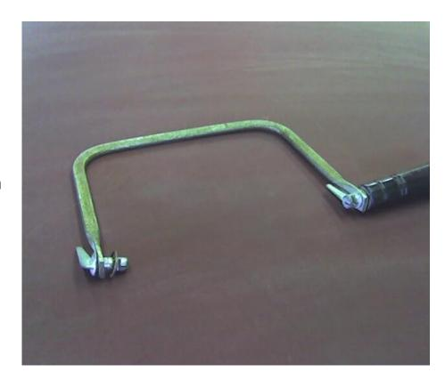
**Step 2.** Remove the end blade attachment, as shown here.
